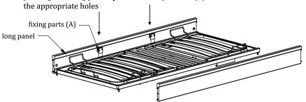
Screw both items (G ) and (H) to the end panels using the screw (C). The markups should help you find the right screwing location.
