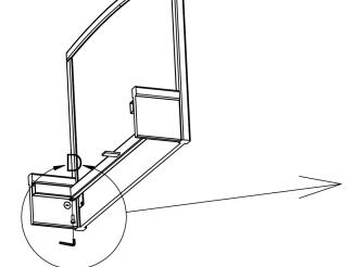
Screw the items (G) and (H) using the screws (F) and the big wrench. Warning: these screws replace the transport screws.
